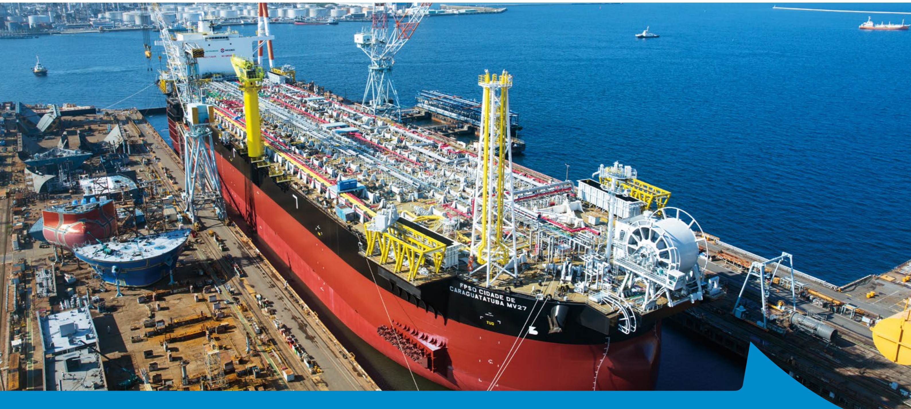
Hull part of a Floating Production, Storage and Offloading Unit ("FPSO Hull")
