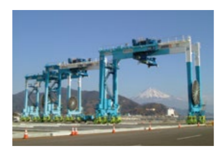
Container Yard Transfer Crane "TRANSTAINER"
