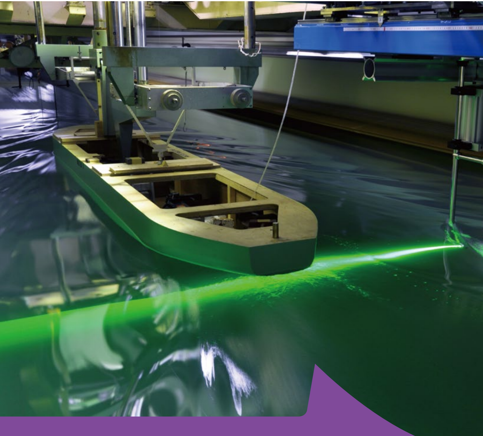
Measuring the flow fields around a ship using a towed PIV device
