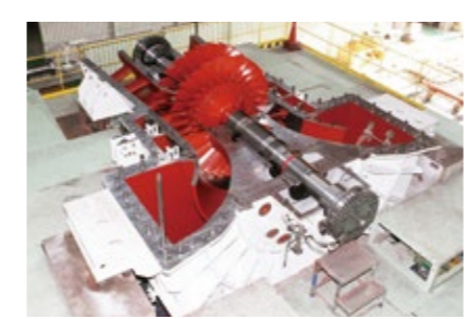
Top Pressure Recovery Turbine
